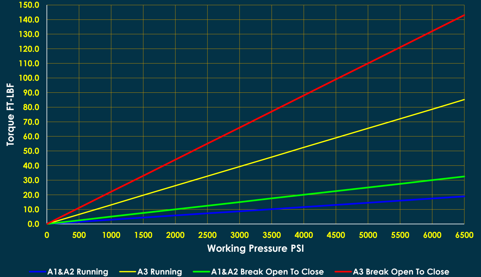
Operating Torque vs Working Pressure
